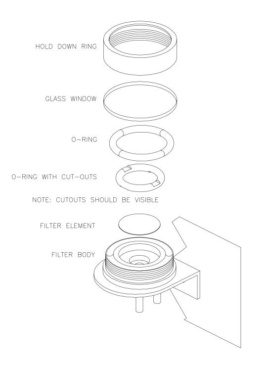
Figure 5.1 - Replacing the Particulate Filter
